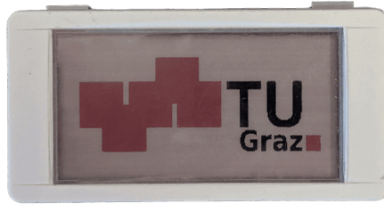
Figure 1.2: A typical node shown in detail, containing a display, a radio transceiver and several other electronic components.
