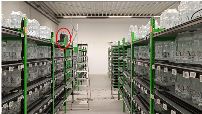
Figure 1.6: The measurement PC is marked in red, which is connected to the SDRs, orchestrating all wideband measurements.
