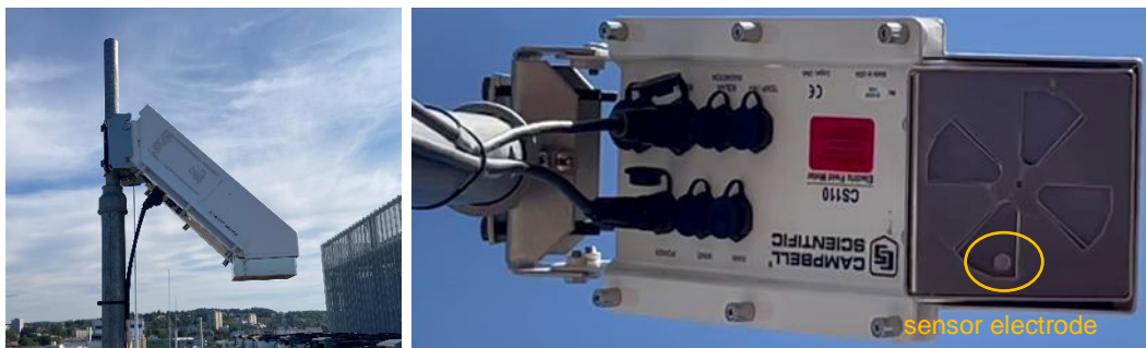
Figure 11: FM-Sensor mounted on tripod (left) and bottom view with open aperture, sensor electrode is visible (right).
