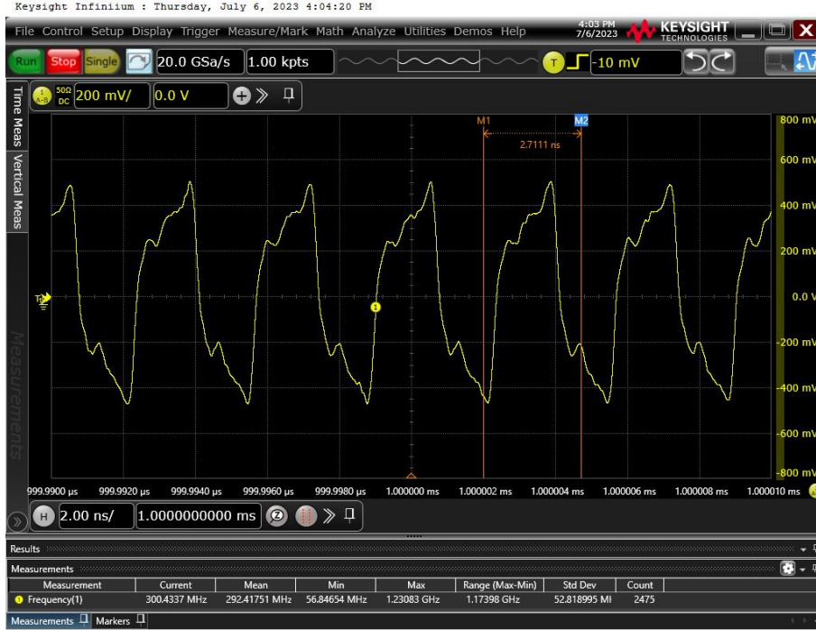
Figure 2.1: Example of a distorted digital signal. 300 MHz clock measured at the receiver input at the end of a 50 cm long fragmented transmission line.
