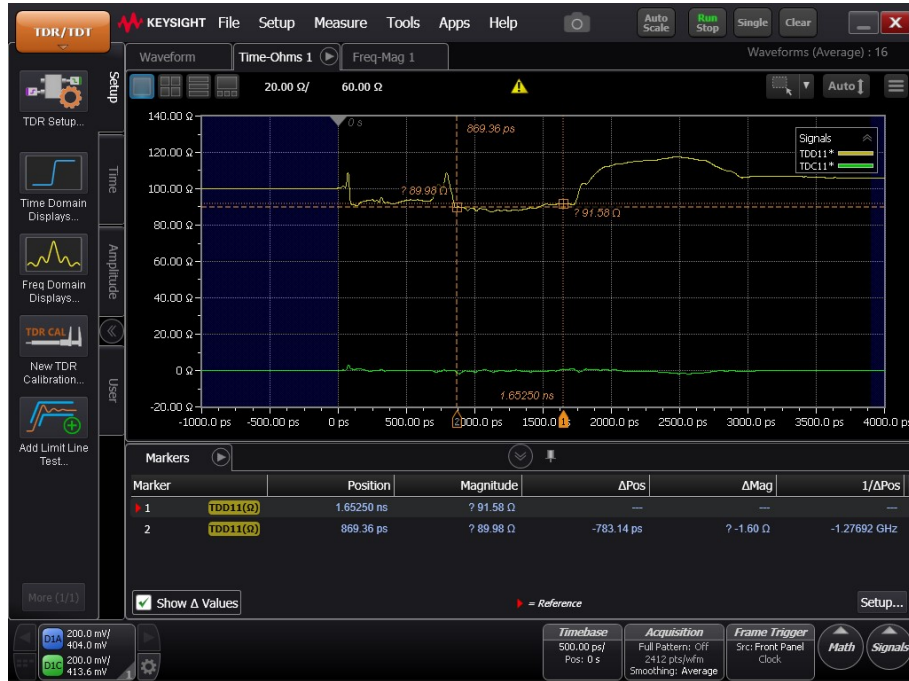
Figure 7.3: Screenshot of the TDR measurement showing the impedance traces for the measurement setup with the IT968 mainboard. The yellow line is the differential impedance, and the green represents the common-mode impedance.
