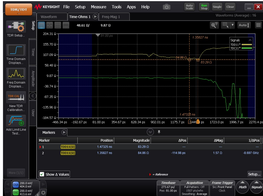
Figure 7.12: Screenshot of the TDR measurement showing the impedance trace for the measurement setup and the FPGAs gigabit receiver.
