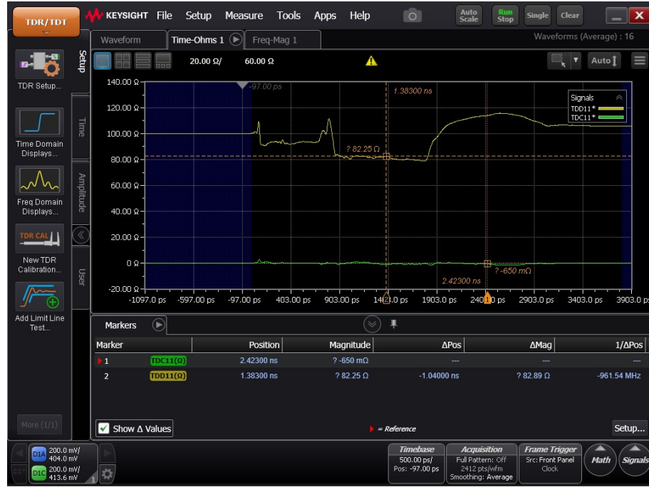
Figure 7.4: Screenshot of the TDR measurement showing the impedance traces for the measurement setup with the IT180-A mainboard. The yellow line is the differential impedance, and the green identifies the common-mode impedance.
