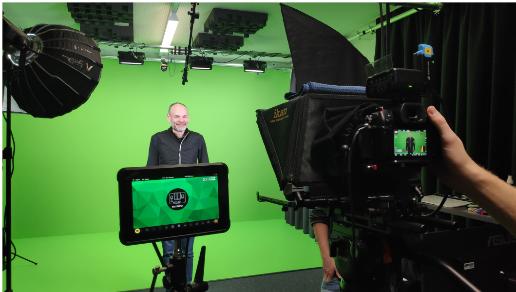
Figure 2.1: Video creation using a Panasonic GH5s camera with Olympus 12-200mm lens with 4k, 25fps, ISO 400, 1/50 shutter speed and 5.6 aperture considering 2m distance to the well-lit green screen and 2m to the front camera.
