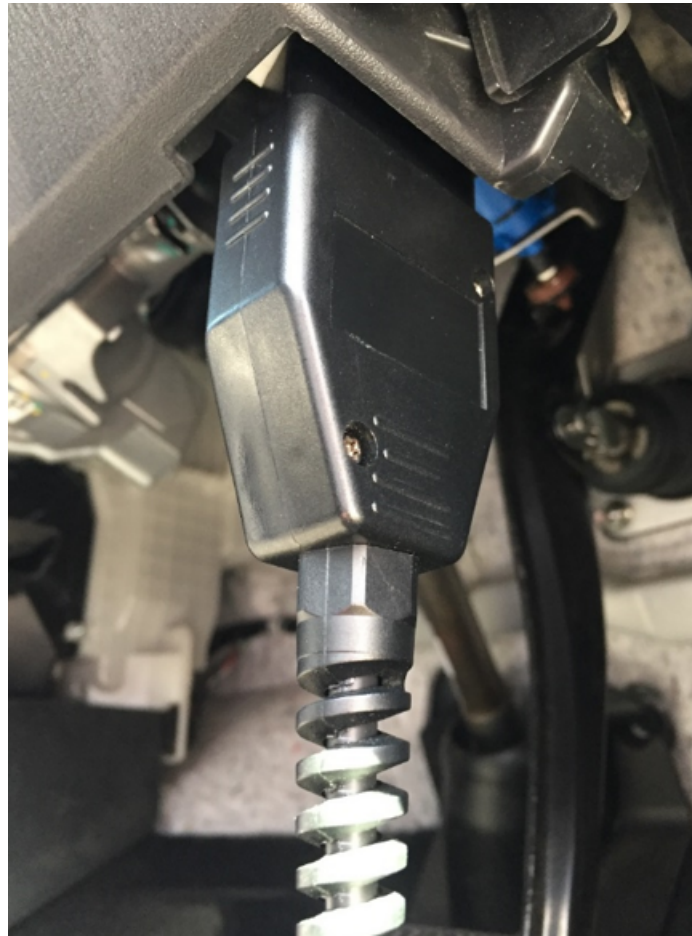
Figure 2.7: Picture of a connected OBD plug in a conventional vehicle
