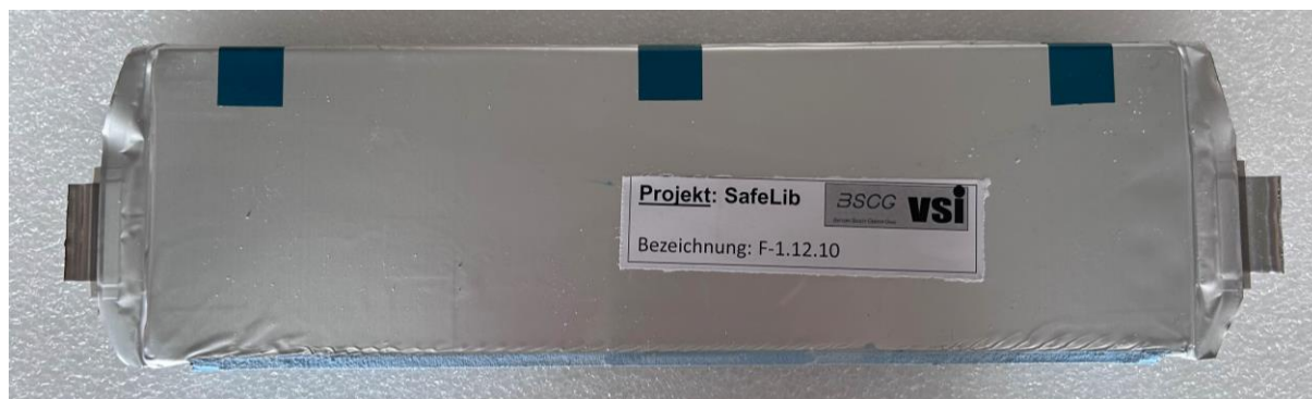
Figure 3.7: Top front view of the lithium ion pouch cell
