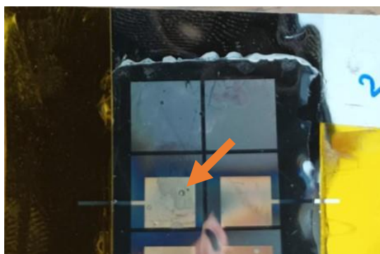
Figure 51. Image of device tested in figure 48, showing electrode corrosion after multiple cycles of humidity exposure
