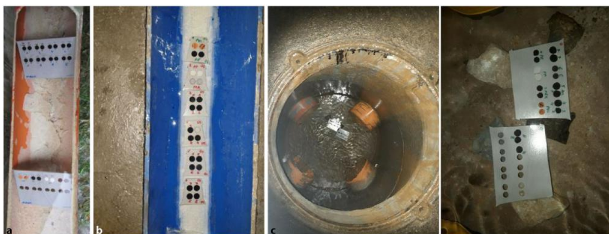
Figure 5: Depositing the plastic samples at the drainage systems of the Steinhaus tunnel (a), Lainzer Tunnel (b) and Zentrum am Berg (c).
