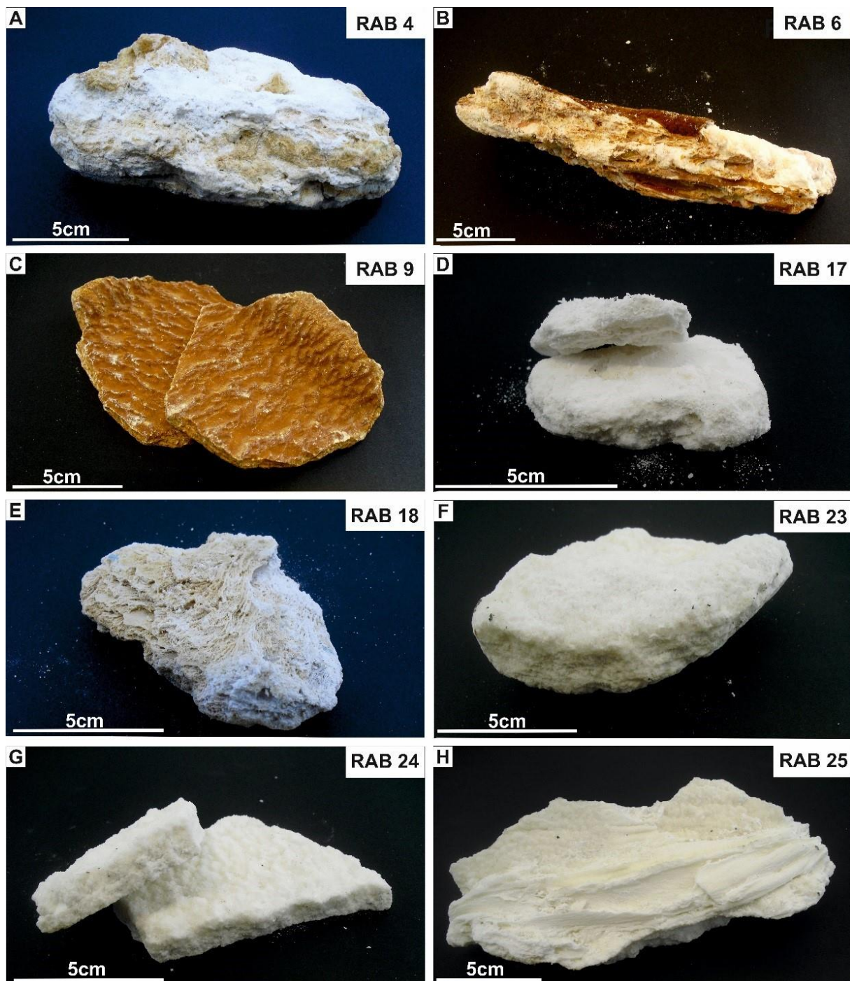
Figure 2: Macroscopic appearance of the scale deposits collected from the motorway tunnel Spital am Semmering (Austria). Specimens RAB 4, 6 and 9 (A, B and C) were sampled from the central drainage channel and display prominent areas of red-brownish coloring, where RAB 9 is rather thin layered and brownish stained (C). Sample RAB 9 is more compact (dense), while RAB 4 and 6 are more porous (A and B). The white colored samples originate from the southern lateral-drainage channel. Precipitates RAB 17, 18 and 25 are highly porous (D, E and H), while the specimens RAB 23 and 24 are more compact (F and G).
