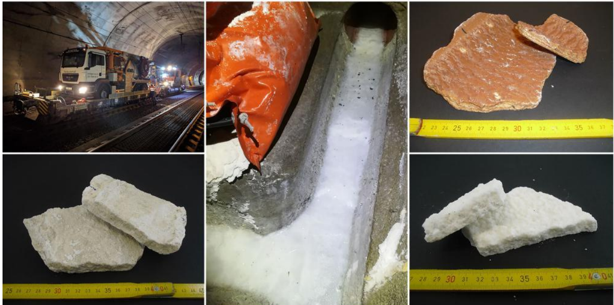
Figure 1: Removal of scale deposits in a railway tunnel and the different visual appearance (e.g. chemical composition, coloring, consistency) of deposits in tunnel drainages.
