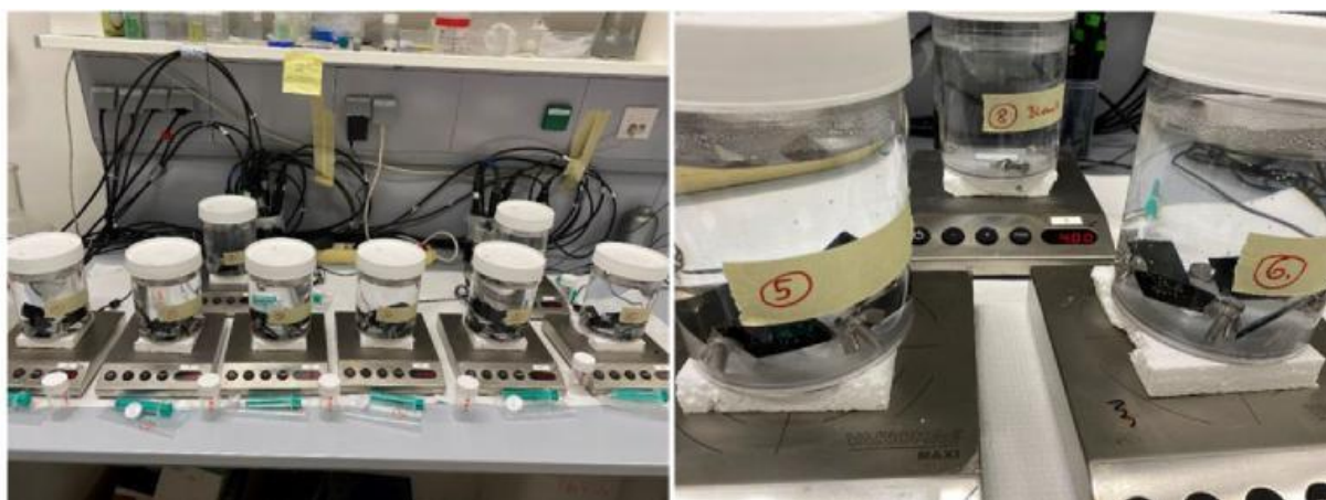
Figure 6: Test reactors for the storage of larger test samples under stationary conditions at the TU Graz.
