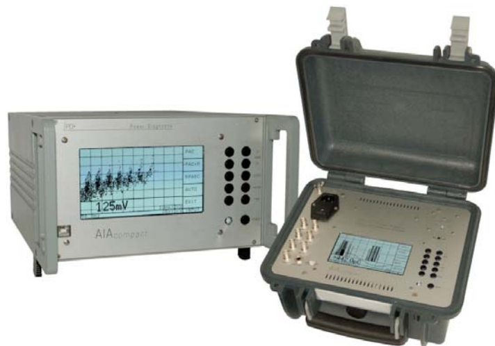
Fig. 5.11 Portable detector for on-site acoustic and UHF spot testing
