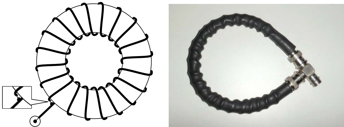
Fig. 4.8 Shielded high frequency Rogowski coil made of thin coaxial cable
