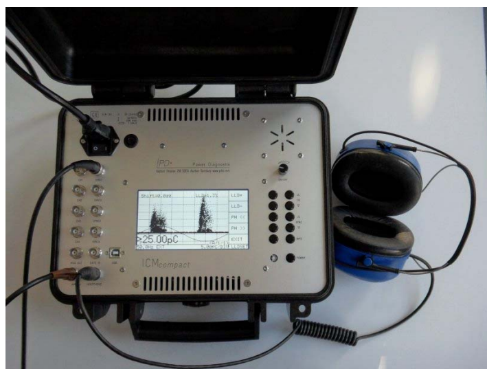
Fig. 6.3 Modern field-test partial discharge detector with speaker and headphone
