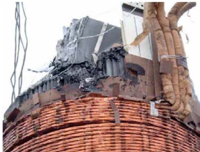
Fig. 7.35 Damage at the located area after failure of the tested unit [57127]
