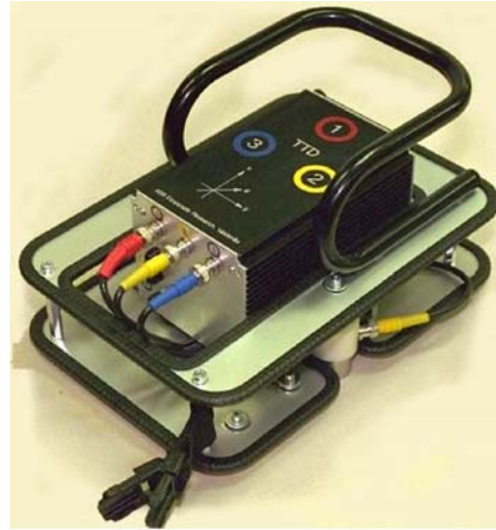
Fig. 7.31 Three-sensor-fixture – sensors evenly spaced by 15cm in a triangle [Ben97]
