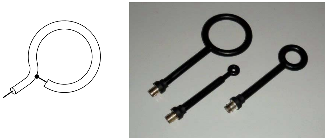
Fig. 4.9 Inductive near field probes (coaxial cable style – principle and examples)
