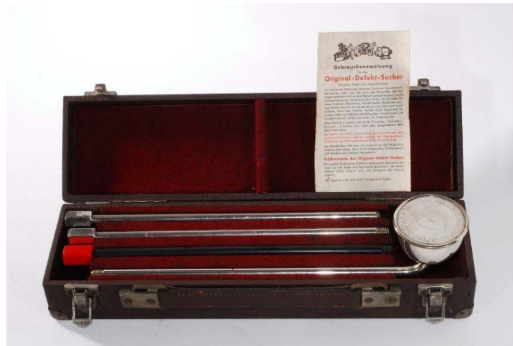
Fig. 4.15 "Original Defekt Sucher", mech. instrument to investigate structural sound (~1930)
