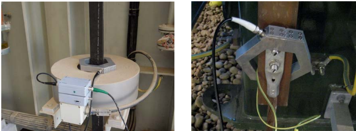
Fig. 7.36 Tapping the neutral connection of a Y-HV (left) and the main ground (right) with a CT
