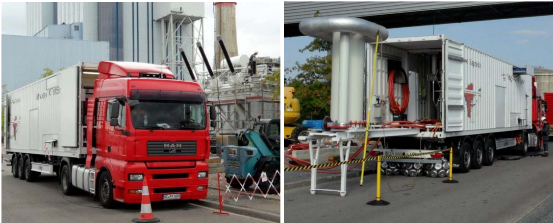
Fig. 7.32 Mobile transformer test system – 500kV, 2MVA series resonant reactor moved out
