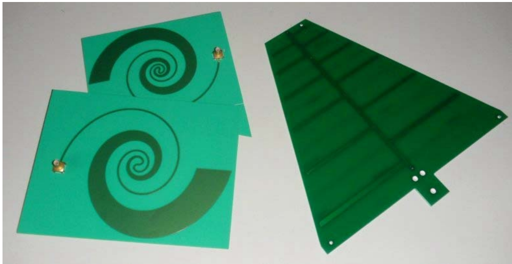
Fig. 4.10 Wideband UHF antennas (left: spiral dipoles 25 , right: log-periodic dipole array)
