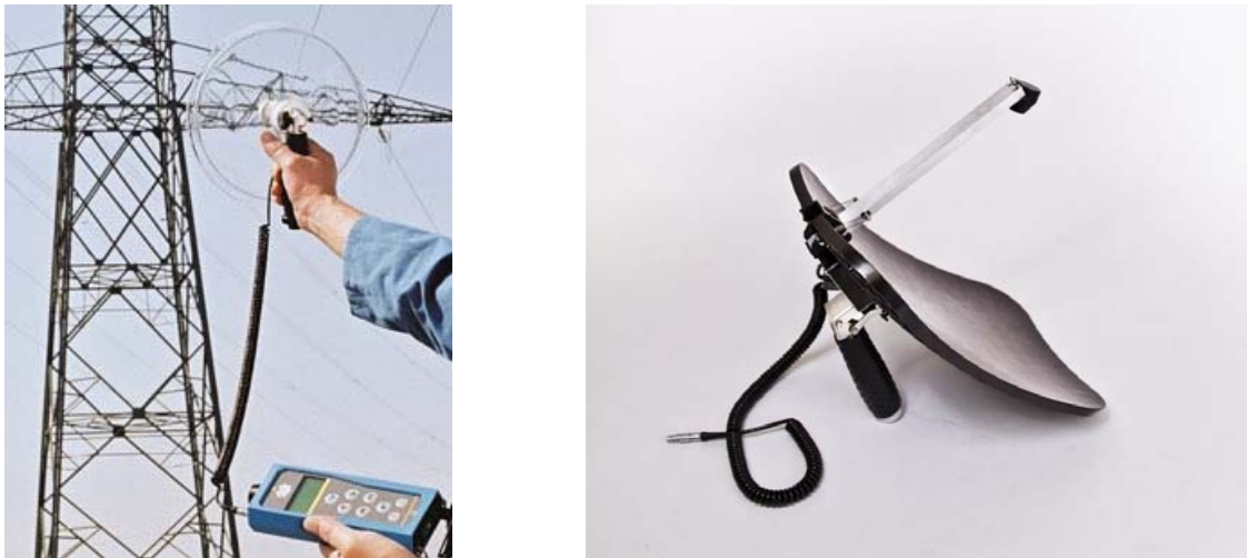
Fig. 4.14 Ultrasonic detection of air-borne partial discharge signal using parabolic reflectors
