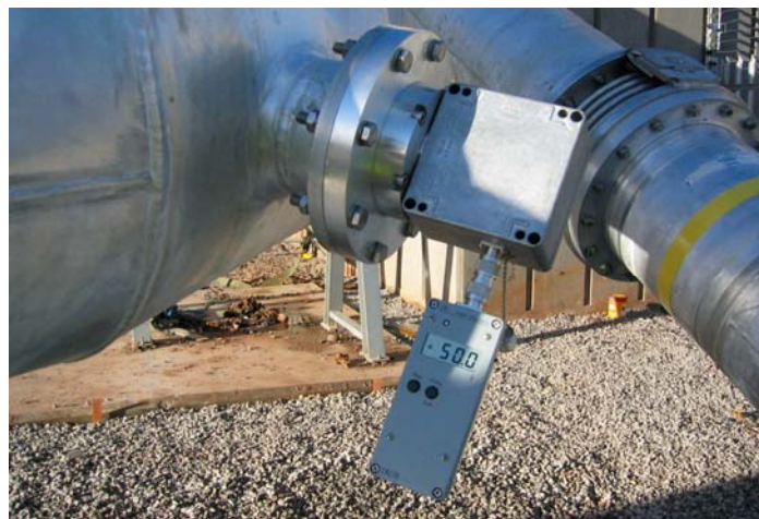
Fig. 3.37 UHF impulse calibrator – injecting step voltage signals with a rise time of <100ps
