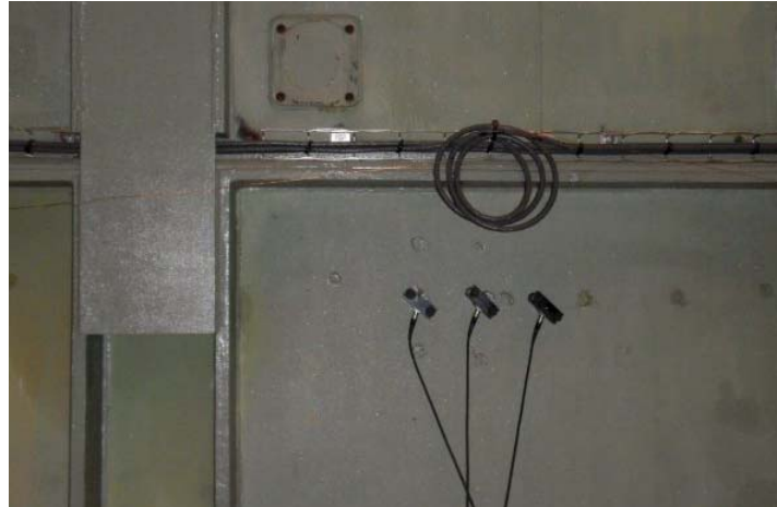
Fig. 7.26 Evenly spaced acoustic sensors to capture the horizontal data
