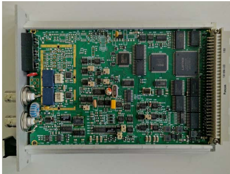
Fig. 5.13 Pre-processing card with spectrum analyzer, 100Msample ADC, and 60270 path
