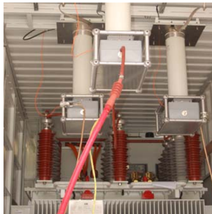
Fig. 7.8 Three high voltage T-filters mounted in a mobile transformer test system
