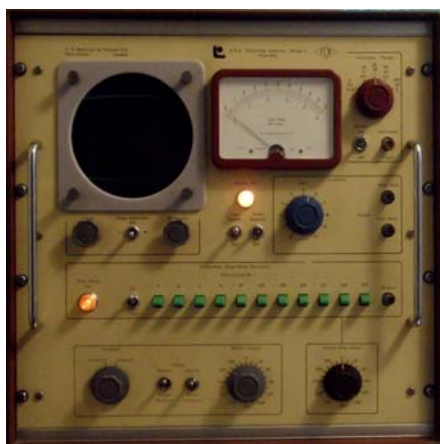
Fig. 6.5 ERA Model 3, early PD detector with Lissajous indication on round CRT screen
