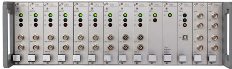
Fig. 7.3 ICMsys8 – eight channel parallel PD and RIV transformer acceptance testing
