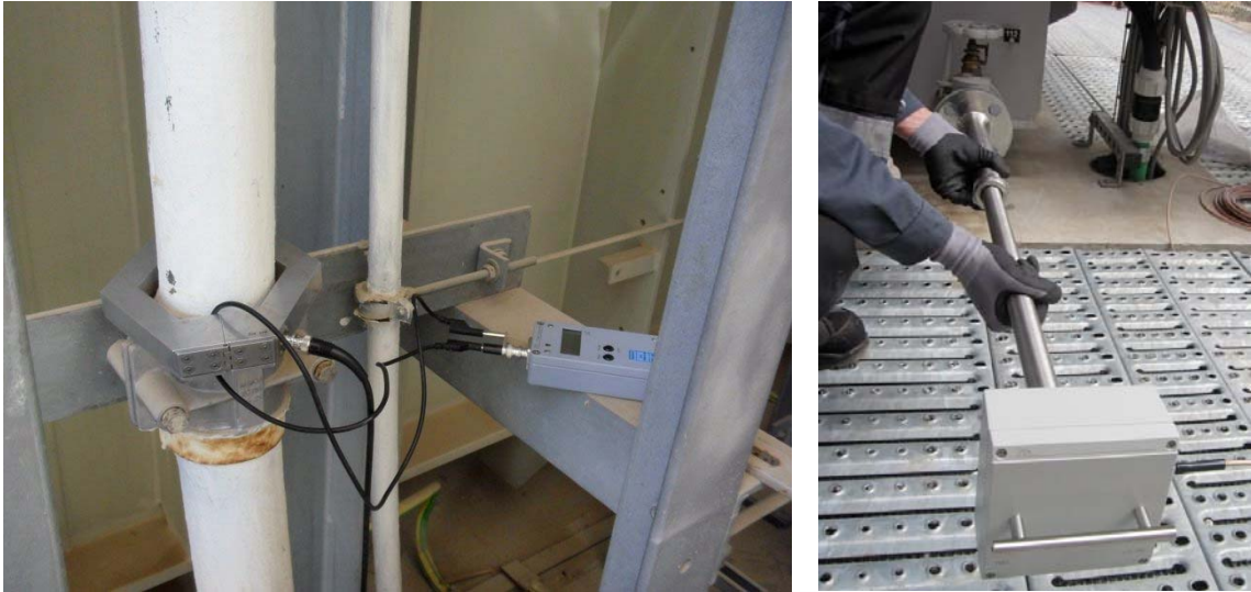
Fig. 7.37 Using a HV cable as coupling capacitor (left) and UHF drain valve sensor (right)
