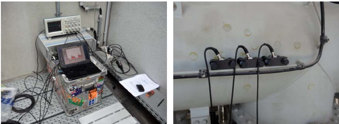
Fig. 7.39 Provisional setup of measurement equipment (left) and acoustic sensors (right)
