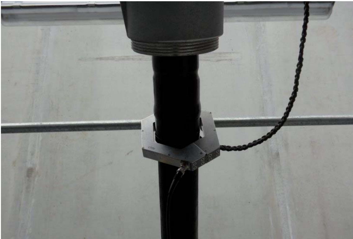
Fig. 4.6 Clip-on RF-CT tapping a 110kV cable to capture transformer PD
