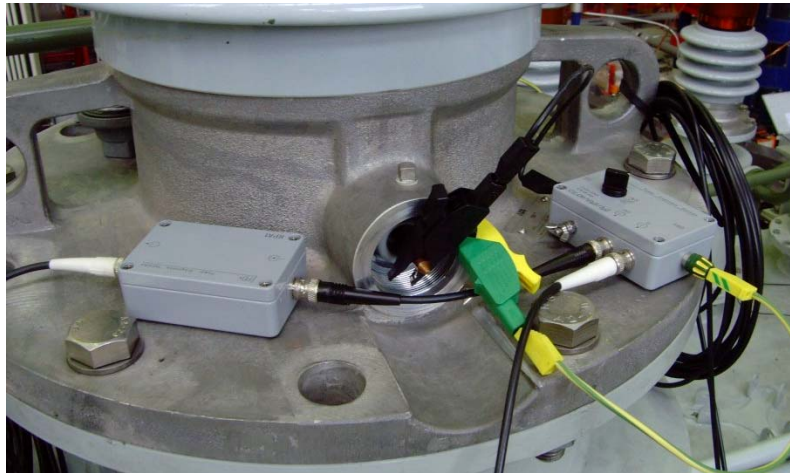
Fig. 7.10 Quadrupole and pre-amplifier connected to a bushing tap
