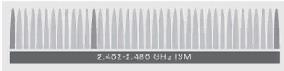
(a) 2.4GHz ISM band with the 2MHz broad channels. The advertising channels are displayed in a darker gray than the data channels.
