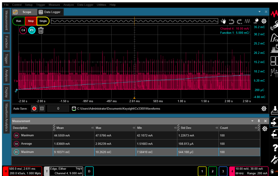
Figure 3.16: Screen capture of the current waveform analyzer used for the charge consumption measurement.
