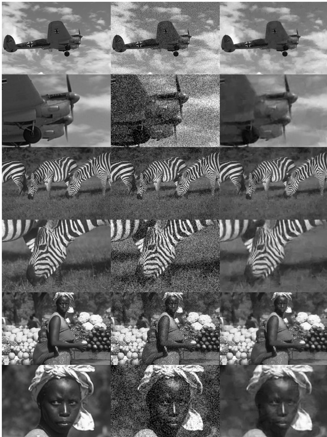
Figure 14: The figure presents a direct comparison between the denoised image (right), the image corrupted with Gaussian noise ( \sigma = 0.1 , middle), and the clean reference image (left), which is sourced from the BSDS500 testing dataset. For detailed inspection, magnified highlights of the full-resolution images ( 481 \times 321 ) are provided below.
