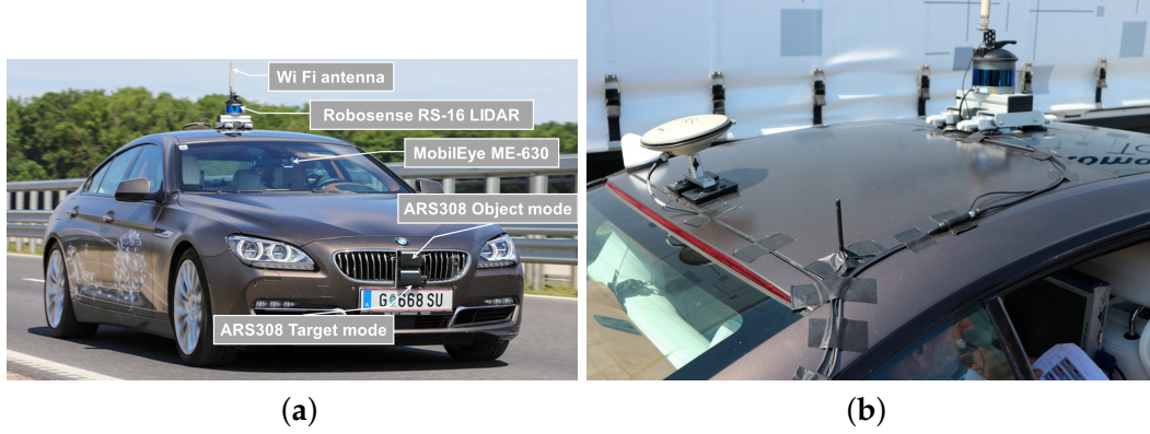
Figure 4.2.: Test vehicle measurement setup. (a) Front view of the test vehicle with the additionally mounted sensors. (b) Top view of the test vehicle with the antennas required.
