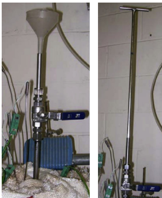
Figure 60: Single valve with funnel (left) and push rod (right) [112]
