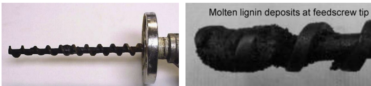
Figure 59: Blocked feed screws caused by molten lignin. left: Bridgewater et al. [112] right: de Wild et al. [88]
