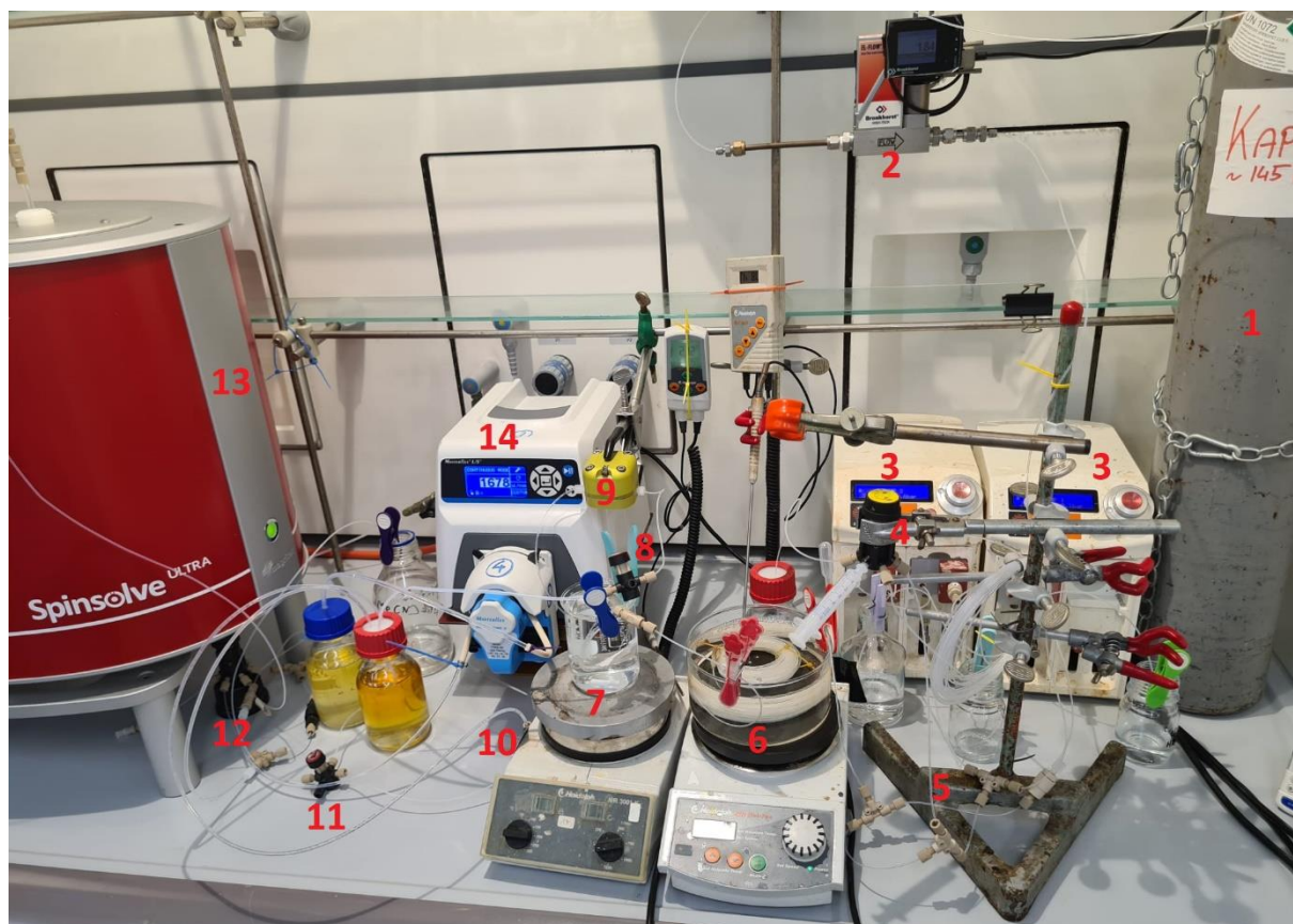
Figure 23. Image of the continuous flow setup for the inclusion of online NMR measurements. 1. oxygen gas cylinder. 2. MFC. 3. syringe pumps. 4. 6-port valve with sample loop. 5. T-pieces. 6. Reactor coil. 7. Cooling coil. 8. 4-port valve for safety pressure release. 9. BPR. 10. T-piece for gas/liquid separation. 11. 4-port valve to flush the flow cell. 12. 6-port valve of the NMR. 13. Benchtop NMR with flow cell. 14. Peristaltic pump.
