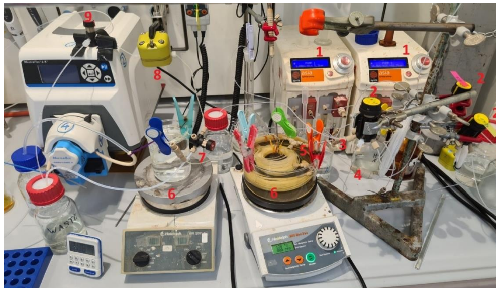
Figure 20. Image of the continuous flow setup: 1. syringe pump, 2. 6-port valve with sample loop to pump the chemicals not directly through the pumps. 3. first T-piece mixed HCl and HNO 3 . 4. tube from the MFC with a check valve 5. T-pieces in the oil bath adding the disulfide feed and the oxygen. 6. reaction coil (right) and cooling coil (left). 7. 4-port valve that can be used to release pressure from the coil in case of clogging. 8. BPR set to 5 bar. 9. 4-port valve for sampling the reaction mixture.
