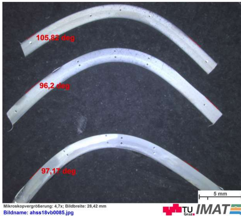
Figure 57 Bending angle after forming of HCT780X at temperatures a) RT b) 500°C c) 900°C
