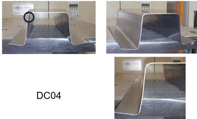
Figure 60 Sidewall curl after forming of DC04
