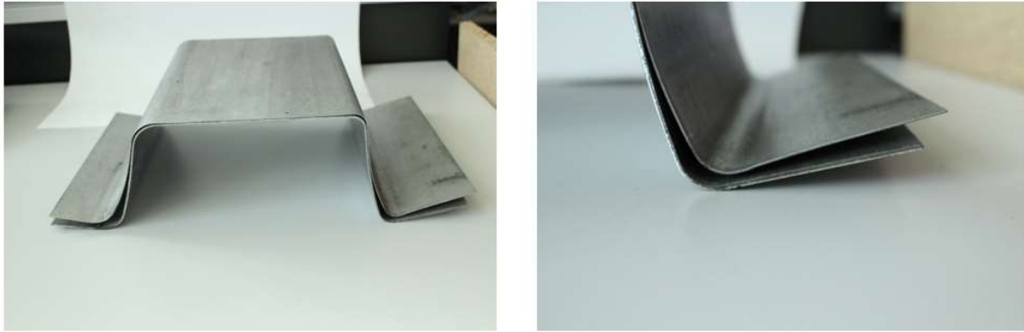
Figure 27 Springback - influence of material thickness at same steel grade
