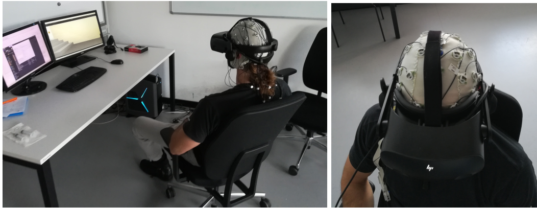
Figure 2.6: The experimental setup, with the EEG cap and the HP Reverb G2 Omnicept Edition VR glasses.
