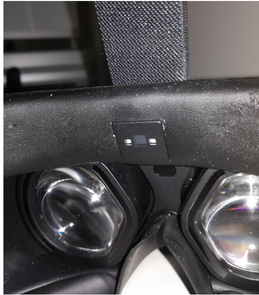
Figure 2.10: The PPG sensor for HR measurement with the 2 green LEDs and the photo-sensor
