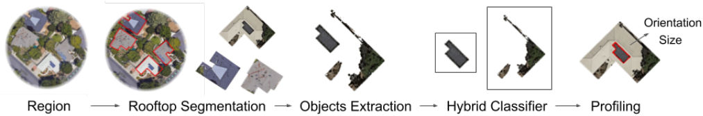
Figure 2.2: SolarFinder processing pipeline. Source: SolarFinder [63]
