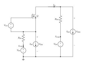
Figure B.4: P-channel MOSFET Circuit-Model with I/O interface.
