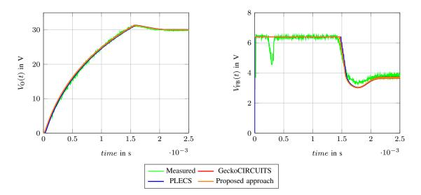
Figure 3.9: Comparison of measurement and simulation results:  $V_{O}(t)$  and  $V_{FB}(t)$  closed-loop flyback converter during start-up.
