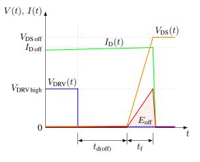
Figure 5.4: Simulated MOSFET switching waveforms during turnoff.
