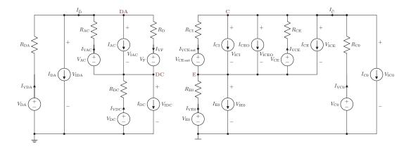
Figure B.10: Universally applicable Optocoupler SubCircuit-Model.
