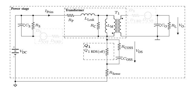
Figure 3.5: Open-loop flyback converter SubCircuit-Model II.
