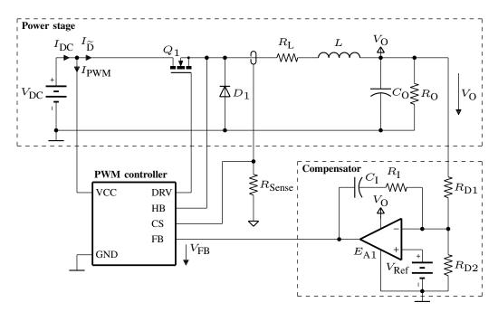
Figure 5.1: Schematic diagram of a closed-loop step down converter with peak current mode control.
