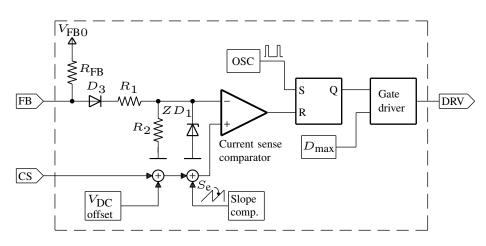
Figure 4.5: Block diagram of the peak current mode PWM controller.
