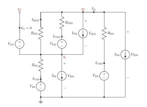
Figure B.5: Universally applicable MOSFET SubCircuit-Model.
