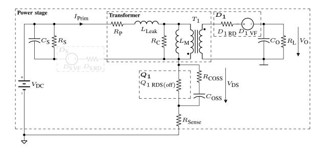
Figure 3.6: Open-loop flyback converter SubCircuit-Model III.
