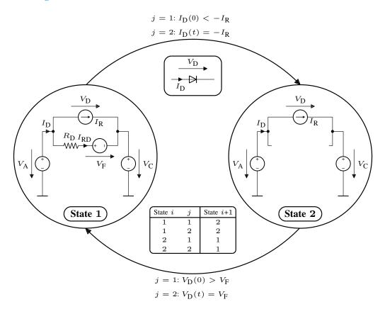
Figure 2.5: Diode state diagram.
