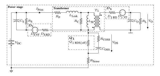
Figure 3.7: Open-loop flyback converter SubCircuit-Model IV.
