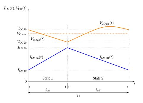
Figure 4.6: Waveforms flyback.
