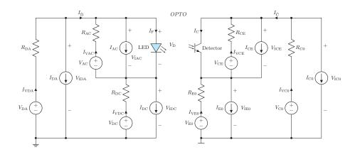
Figure B.9: Optocoupler Circuit-Model with I/O interface.
