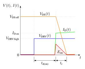
Figure 5.3: Simulated MOSFET switching waveforms during turnon.
