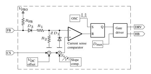
Figure 5.2: Block diagram of the peak current mode PWM controller.
