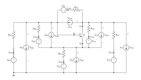
Figure B.6: NPN BJT Circuit-Model with I/O interface.
