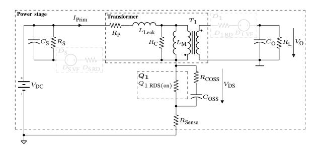
Figure 3.4: Open-loop flyback converter SubCircuit-Model I.
