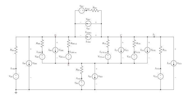
Figure B.8: Universally applicable BJT SubCircuit-Model.
