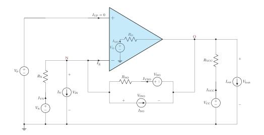
Figure B.12: Universally applicable amplifier SubCircuit-Model.
