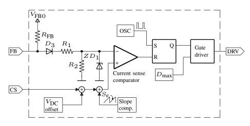
Figure 3.3: Block diagram of the peak current mode PWM controller.
