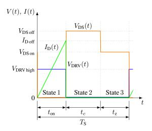
Figure 5.6: Simulated MOSFET switching waveforms for one switching period  $T_{\rm S}$  in DCM.<sup>4</sup>
