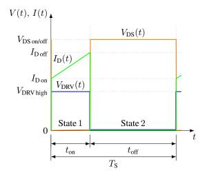
Figure 5.5: Simulated MOSFET switching waveforms for one switching period  $T_S$  in CCM.
