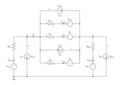
Figure B.2: Universally applicable diode SubCircuit-Model.
