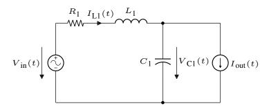
Figure 4.1: SubCircuit-Model: RLC series resonant circuit.
