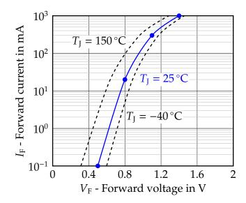
Figure 1.1: Illustrated forward voltage characteristic for different junction temperatures  $T_{\rm J}$  of a GP diode.
