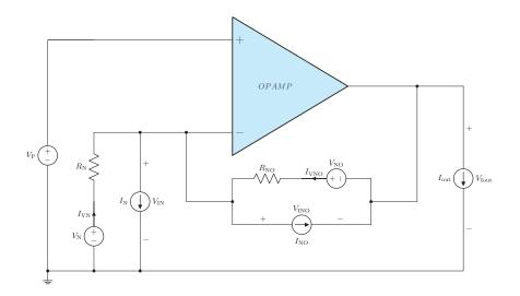
Figure B.11: Amplifier Circuit-Model with I/O interface.
