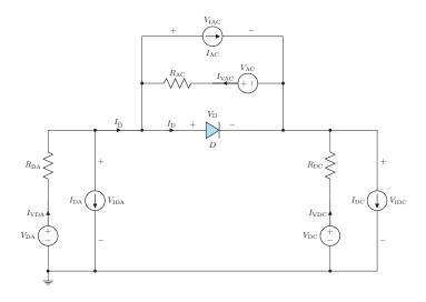
Figure B.1: Diode Circuit-Model with I/O interface.
