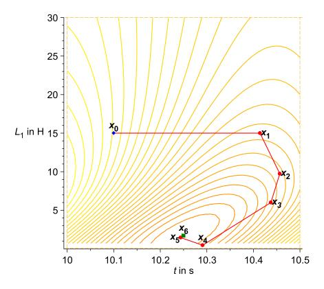
Figure 4.3: RLC series resonant circuit contour plot  $I_{L1 max function}(t, L_1)$ .
