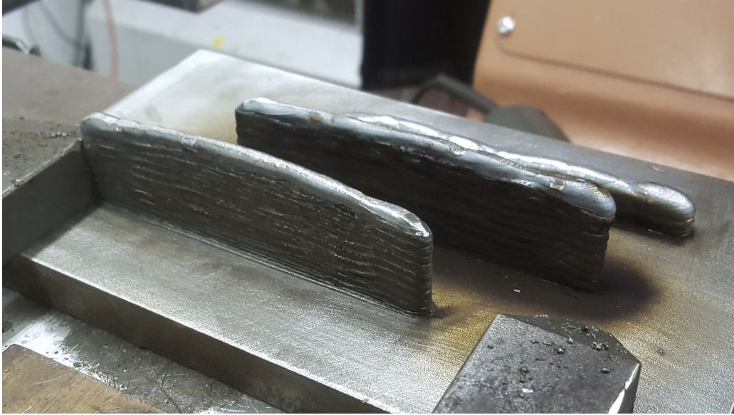
Figure 5.10: Results of the controlled (middle) and uncontrolled (foreground) single bead multi layer experiment with alternating weld direction. The small wall in the background is a test run for the desired layer height \Delta z .
