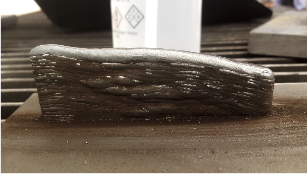
Figure 5.5: Result of the controlled single bead multi layer experiment. For details on the geometry see figure 5.4
