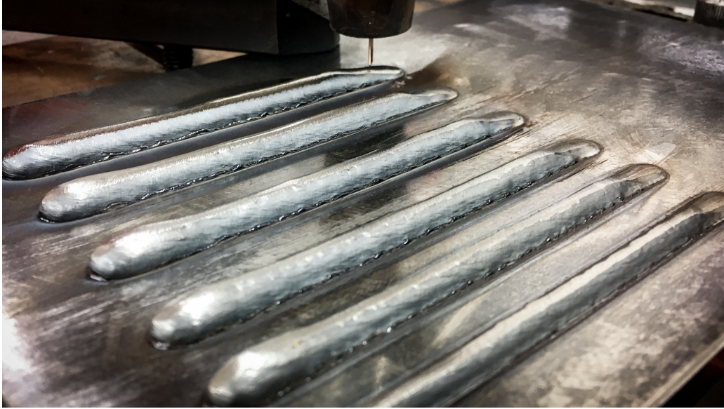
Figure 5.1: Two layers for each of the 5 different tested travel speeds. One trial was redone, therefore there are six beads.
