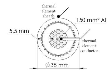
Figure 6-9: Position of the thermal elements in the cable
