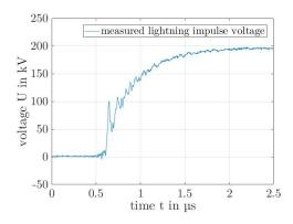
Figure 5-12: Measured lightning impulse voltage with low voltage part B
