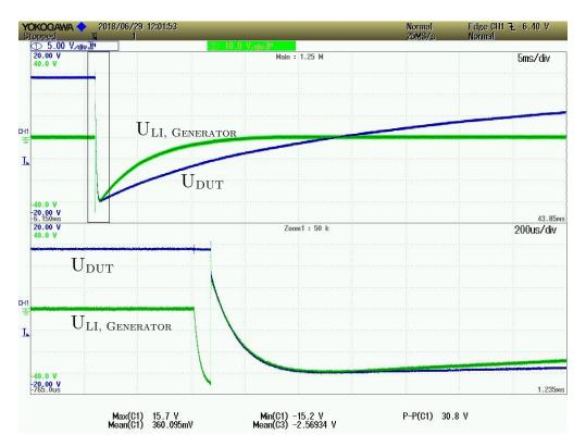
Figure 6-12: Problem when using spark gap as coupling element (bottom: zoomed)
