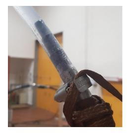
Figure 6-10: Water resistor, conical shaped plug
