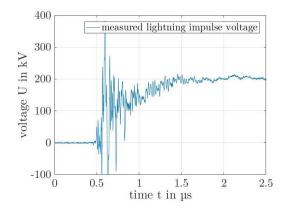
Figure 5-8: Measured lightning impulse voltage with low voltage part A
