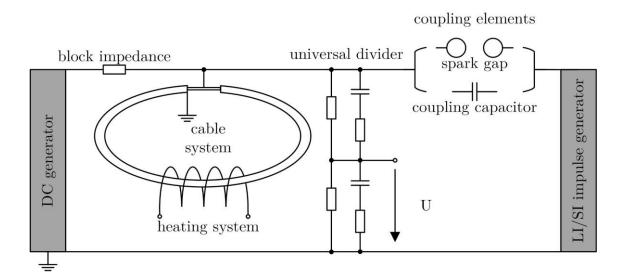
Figure 4-3: Scheme of the test setup
