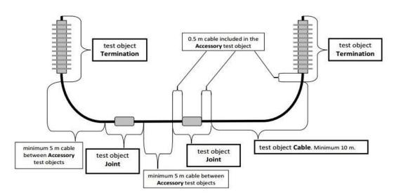
Figure 4-1: Example of a test loop according to TB 496 [25]
