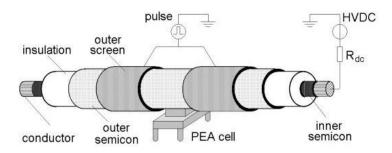
Figure 2-9: Measurement setup for PEA with a cable [21]
