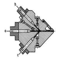
Figure 2-3: Schematic drawing of a triple extrusion [14]
