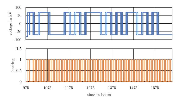
Figure 7-5: Voltage and current over time for load cycle with polarity reversal (LC + PR)
