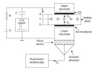
Figure 2-8: Block diagram of the pulsed electroacoustic (PEA) method [13]
