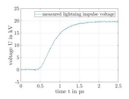
Figure 5-13: Measured lightning impulse voltage (impulse from HILO)
