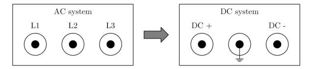
Figure 7-9: Cable system conversion
