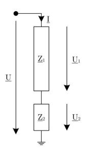
Figure 5-2: Voltage divider with two impedances
