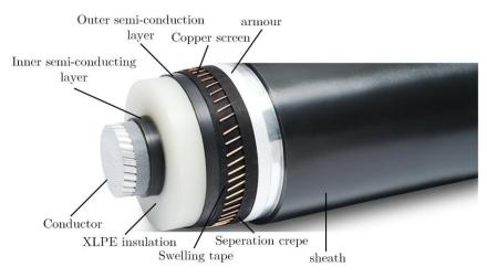
Figure 2-2: Typical extruded MVAC cable [15]
