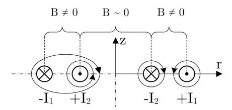
Figure 5-21: Magnetic flux situation by using double helix design
