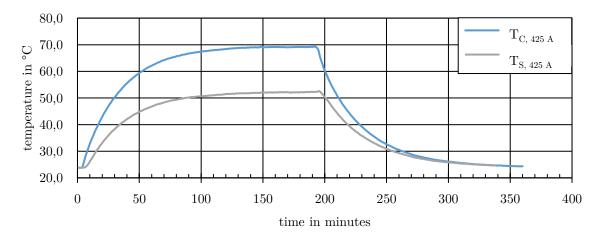
Figure 7-1: Temperature development over the time, I = 425 A
