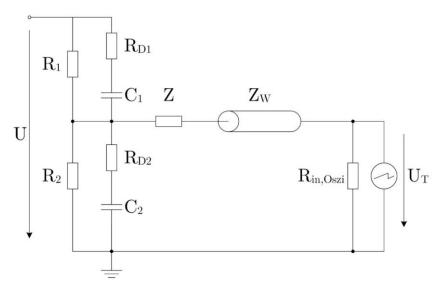
Figure 5-3: Simplified circuit of a universal voltage divider
