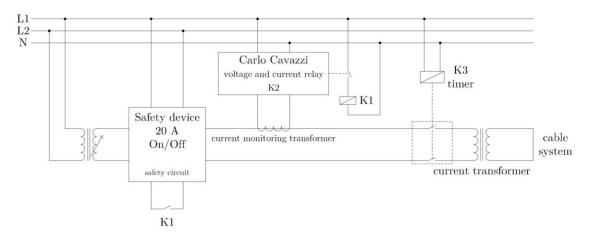
Figure 6-7: Current circuit with safety circuit
