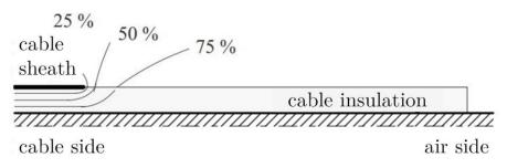
Figure 6-2: Electrical field distribution at end of a cable, uncontrolled [3]
