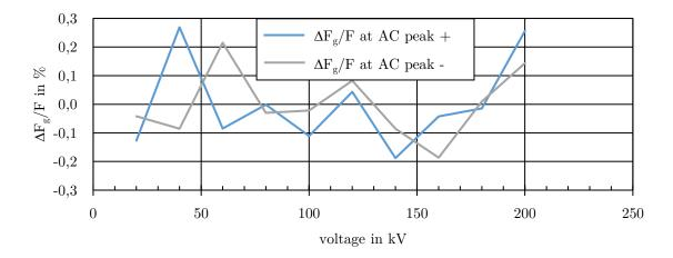
Figure 5-19: Relative change of scale factor over the voltage, AC
