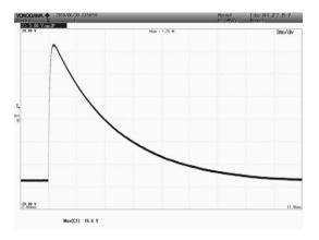
Figure 7-6: S/IMP with + 55 kV DC and - 65,6 kV SI
