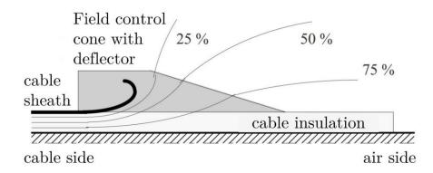
Figure 6-3: Electrical field distribution at end of a cable with geometrical field control [3]
