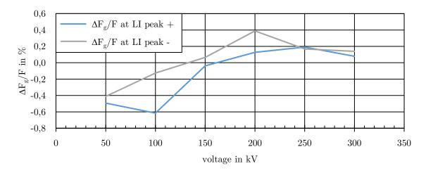
Figure 5-20: Relative change of scale factor over the voltage, LI
