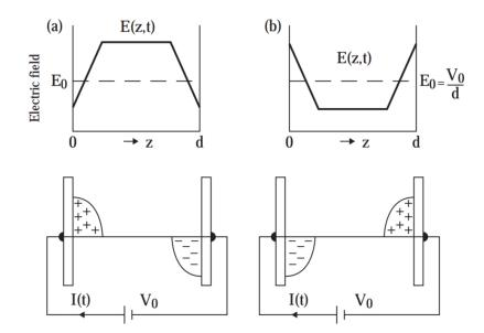
Figure 2-5: Electric field distribution [13] a) homocharge b) heterocharge
