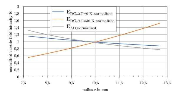
Figure 2-4: Electric field density E over the radius r
