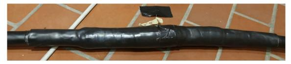
Figure 6-5: Installed standard 12/20 kV AC cable joint
