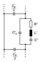
Figure 5-4: Simplified equivalent circuit of capacitive divider with concentrated earth capacity [32]
