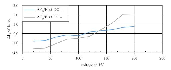
Figure 5-18: Relative change of scale factor over the voltage, DC
