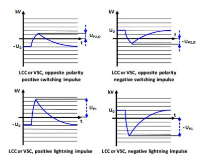
Figure 4-2: Superimposed test voltages according to Cigré TB 496 [25]
