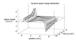
Figure 2-10: Dynamic space charge distribution over time [21]
