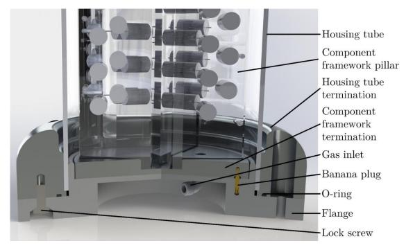
Figure 5-26: Sectional view of bottom of the universal divider
