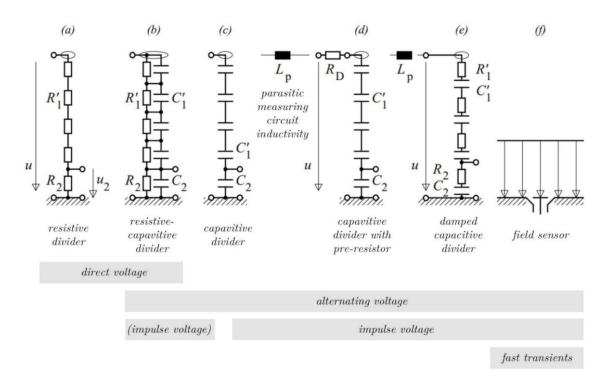
Figure 5-1: Different types of high voltage dividers [3]
