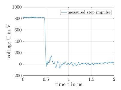
Figure 5-14: Step response of high voltage divider
