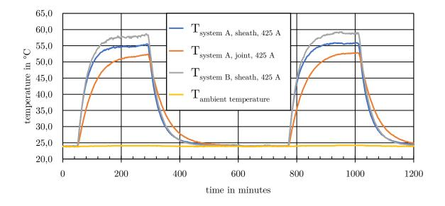
Figure 7-2: Temperature development over time during short Load Cycle (LC)
