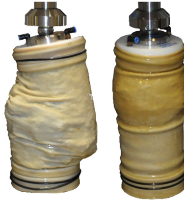
Fig. 2: Specimens after shearing, left: unreinforced, right: reinforced
