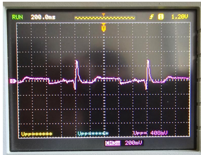
Figure 54: Measurement of the Einthoven lead 3
