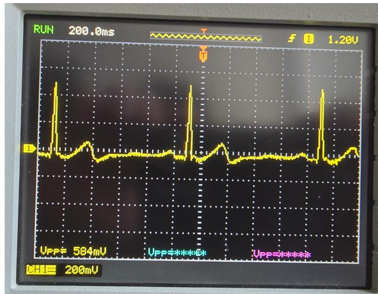
Figure 52: Measurement of the Einthoven lead 1
