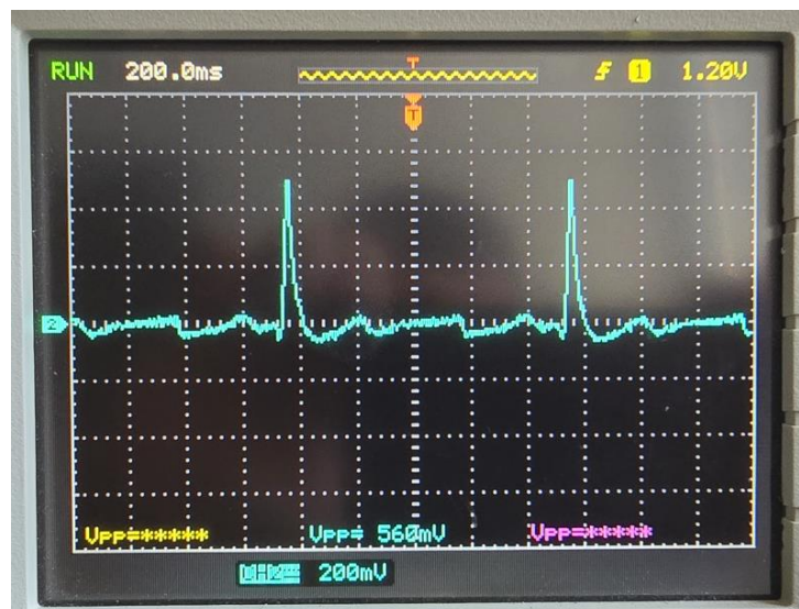
Figure 53: Measurement of the Einthoven lead 2
