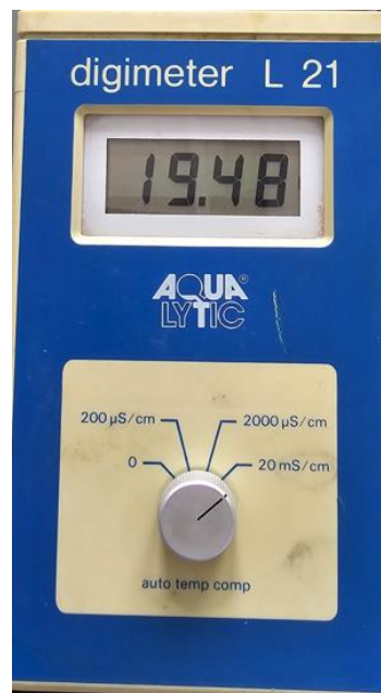
Figure 40: Instrument for the conductivity of the electrolyte
