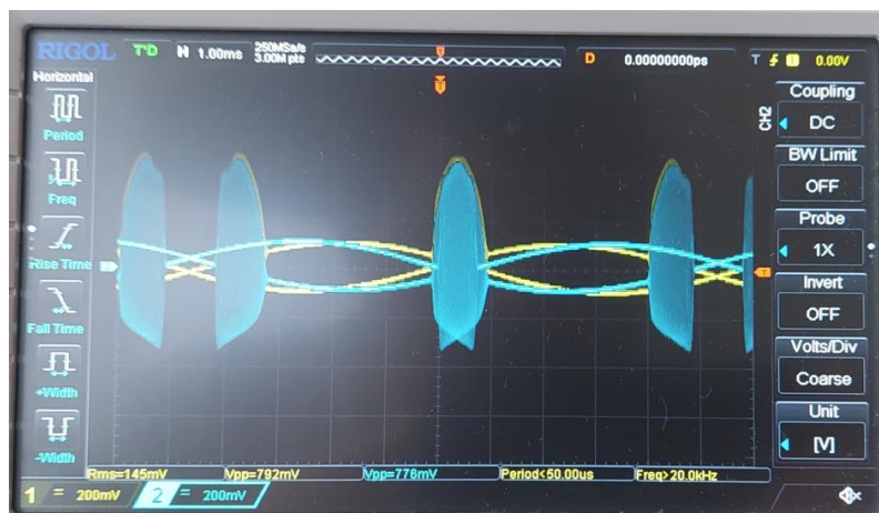
Figure 18: Stability problems LM358
