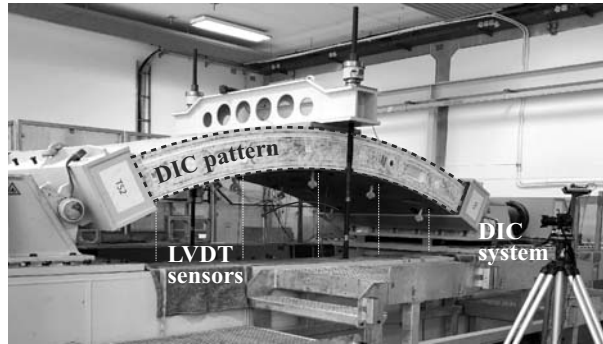
Figure 6.11: Test rig for real-scale tunnel lining segments (based on Monsberger and Lienhart 2021b).
