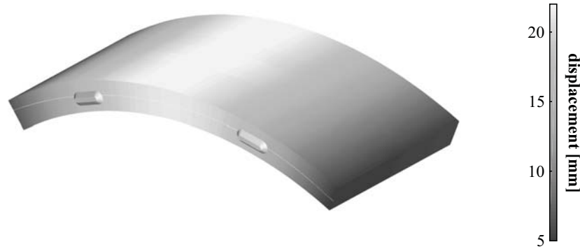
Figure 6.13: Areal displacement map of tested tunnel segment derived from DFOS at highest load step (Monsberger and Lienhart 2021b).
