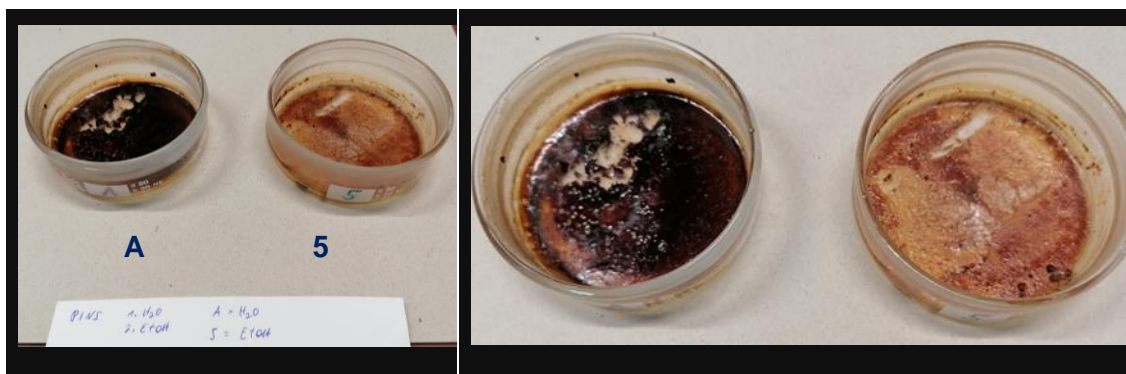
Figure 43_ Evaporated residual solids from Soxhlet extraction according to NREL LAP 42619 of a spruce sample (first H 2 O, then EtOH); beaker A (left) was the residue from the water extraction and beaker 5 (right) contains the residue from the ethanol extraction
