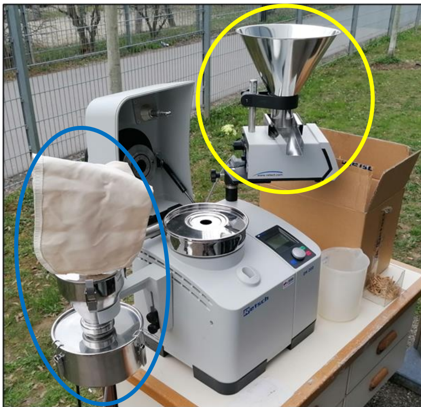
Figure 37_Picture of an open RETSCH ultra centrifugal mill ZM 200 with accessories in circles; yellow circle a DR 100 vibration distribution device (used for even, continuous dispensing and conveying of free-flowing bulk materials and fine powders); blue circle a cyclone with dust filter and stainless-steel collection container
