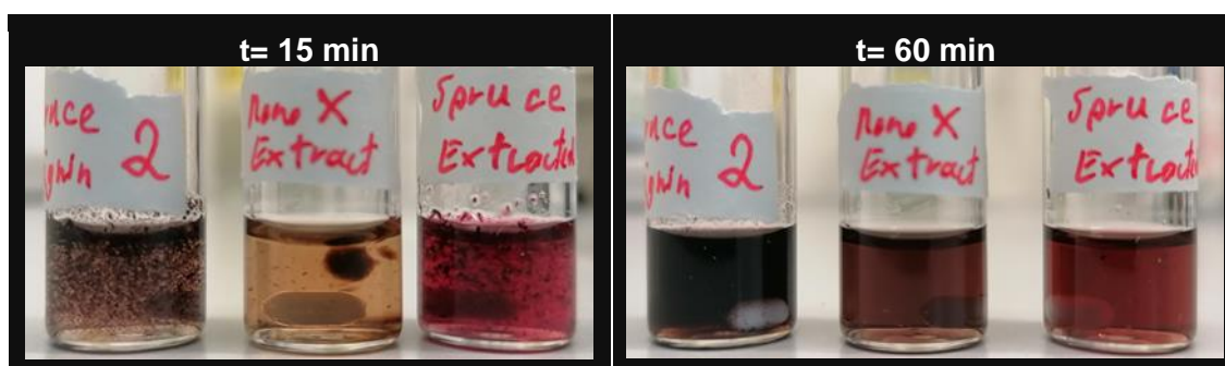
Figure 80_Sample of how the total lignin interferes with the color reaction of the carbohydrates; shown from left to right, spruce Klason lignin fraction, MonoX (extracted) and a spruce sample (extracted)
