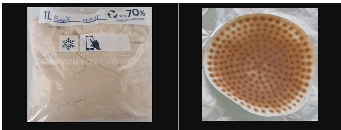
Figure 41_For comparison a picture of the Klason lignin determination step of a full pretreated pulp sample and their filter disk residues, showing no residues of incomplete hydrolysis
