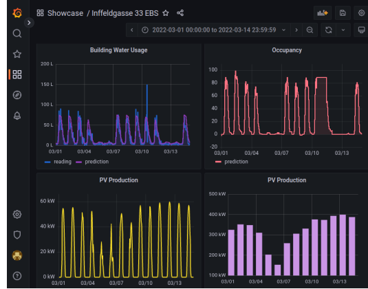
Figure 6.5: A Grafana dashboard. This showcase example visualizes predicted and actual water consumption, predicted occupancy as well as predicted hourly PV production and actual daily PV production.
