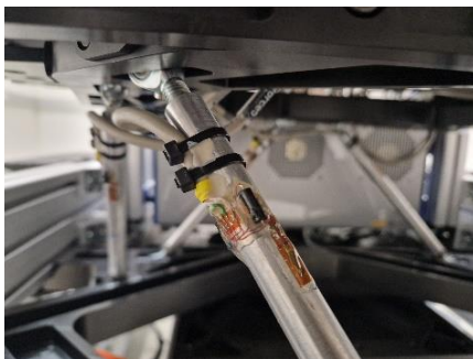
Figure 2- 39: (left) Example of sensor installed on hexapod rod; (right) Example of hexapod rods indication on hardware, clockwise
