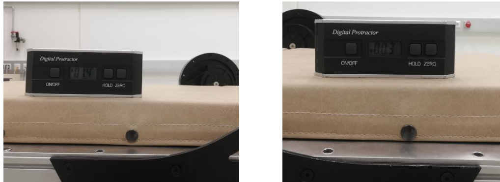
Figure 2- 65: Seat angles, (left) Seatback, (right) Seat cushion
