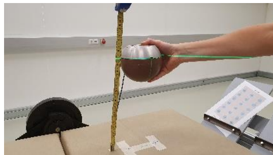
Figure 3- 22: Freefall child head impactor
