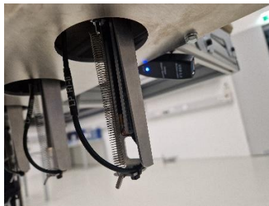
Figure 2- 37: Example of potentiometer in seat foam
