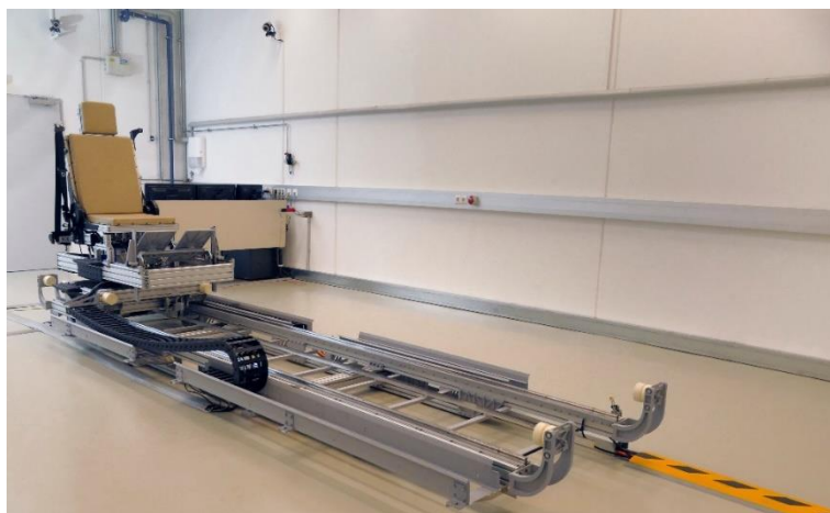
Figure 1- 2: Sled testbed LowG
