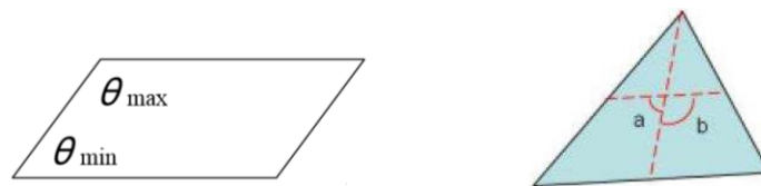
Figure 2- 49: Skewness angle (left) hexa/quad elements [22] ; (right) tetra/tri elements [23]
