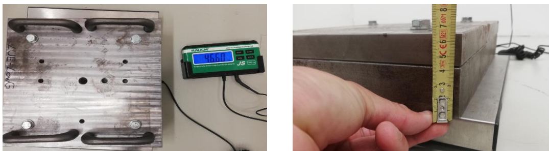
Figure 2- 63: Steel plate used as ballast (left) Weight measure; (right) Thickness measurement
