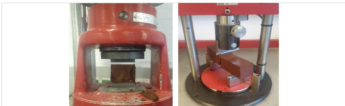
Figure 8 Compressive strength (left) and tensile strength test (right) of BA1
