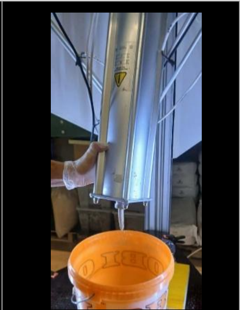
Figure 13 Extrudability test of HM4
