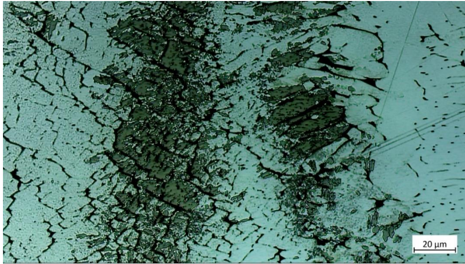
Figure 39: Microstructure of EBW melted AISI 304L, hot compressed at temperatures of 950°C and a strain rate of 1 s -1 , wet etched with Beraha 2
