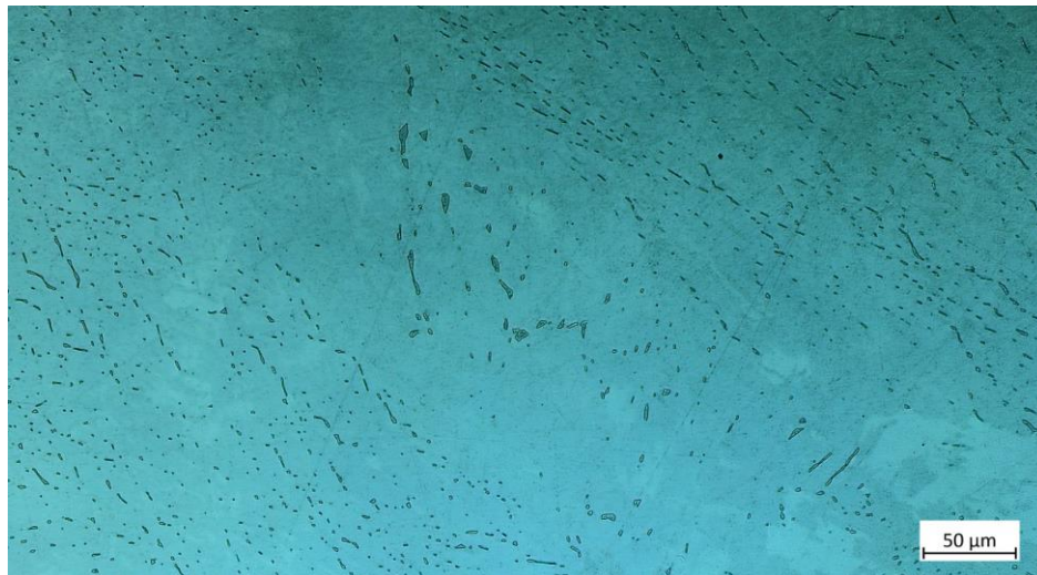
Figure 46: Globularized microstructure of EBW melted AISI 304L, hot compressed at temperatures of 1100°C and a strain rate of 0.001 s -1
