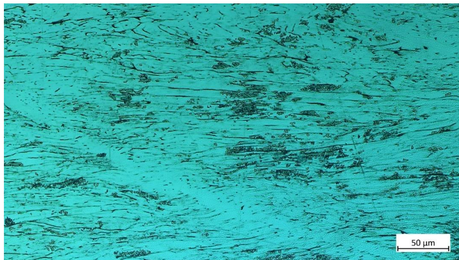
Figure 26: Microstructure of EBW melted AISI 304L austenitic stainless steel after hot compression at 800°C and a strain rate of 0.1 \text{ s}^{-1} and wet etching with Beraha 2
