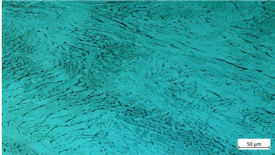
Figure 48: Microstructure of EBW melted AISI 304L, hot compressed at temperatures of 900°C and a strain rate of 0.001 s -1 , wet etched with Beraha 2
