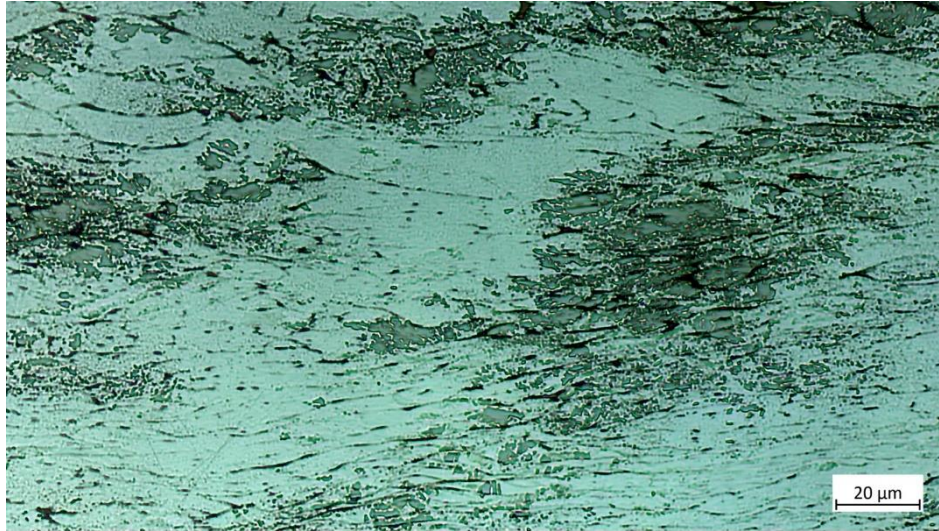
Figure 37: Microstructure of EBW melted AISI 304L, hot compressed at temperatures of 800^\circ\text{C} and a strain rate of 0.01\text{ s}^{-1} , wet etched with Beraha 2 showing poor visibility of the \delta -ferrite phase
