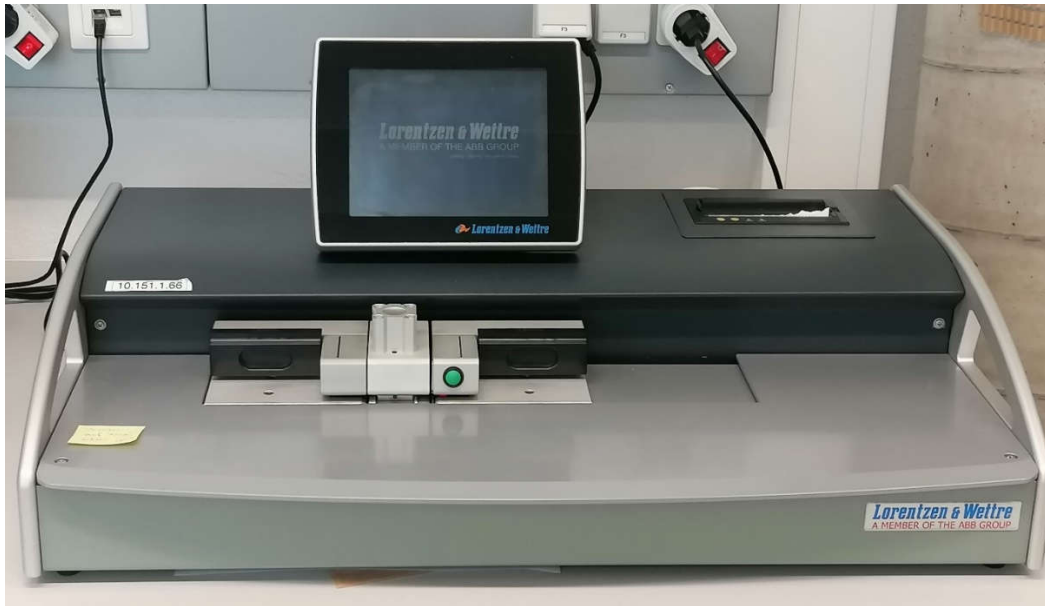
Figure 4-4: Measuring instrument from L&W for the notched tensile test.
