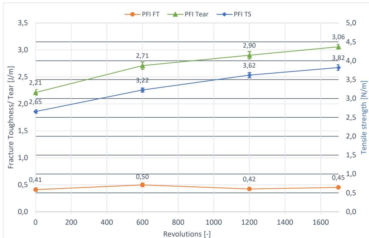
Figure 5-9: Fracture toughness, tear, and tensile strength of lab PFI refining
