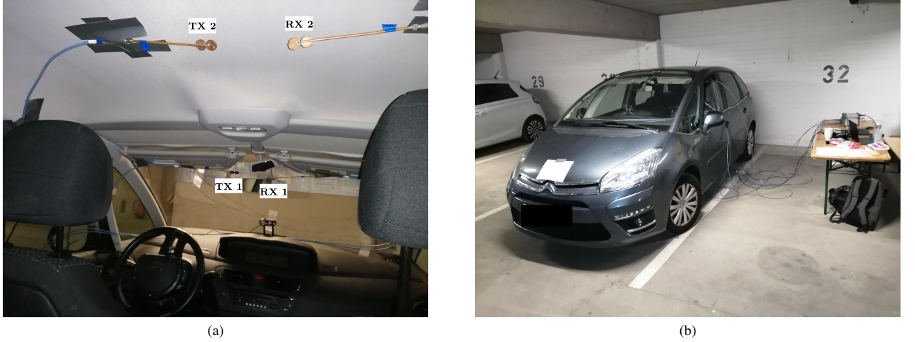
Fig. 2: Antenna placement inside the Citroen Picasso (a) and the environment around the car (b).
