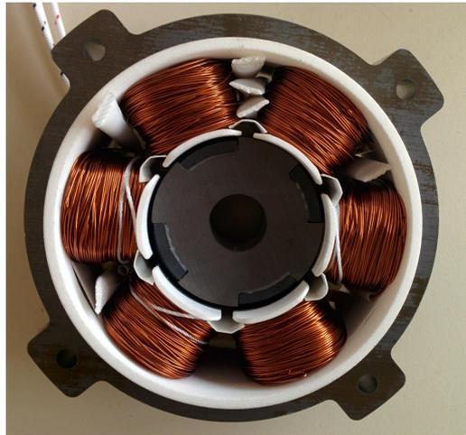
**Fig. 9:** PMSM prototype.
